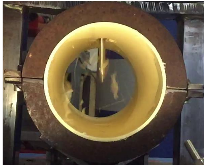
Figure 12. The PVC-U pipe segment fails in a brittle way when a smaller striker is used at 5 °C (compare with Figure 10).
