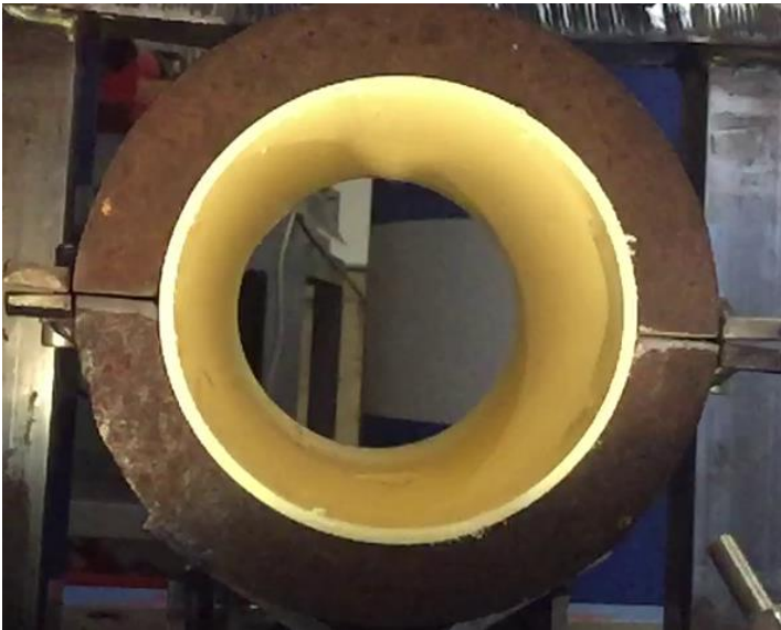
Figure 11. Still made with a high-speed camera just before failure. As at room temperature, there is hardly any local deformation of the PVC-U pipe segment at 5 °C around the small striker (Figure 9).
