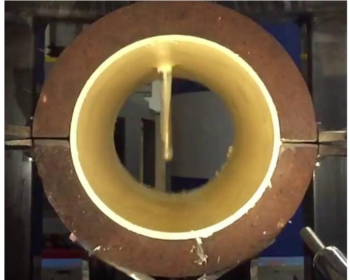
Figure 10. The PVC-U pipe segment fails in a ductile way when a smaller striker is used (compare with Figure 6).
