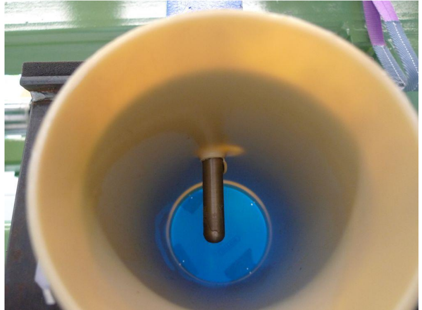
Figure 8. A different PVC-U pipe failed in a ductile way, when the test parameters were exactly the same as in Figure 7.
