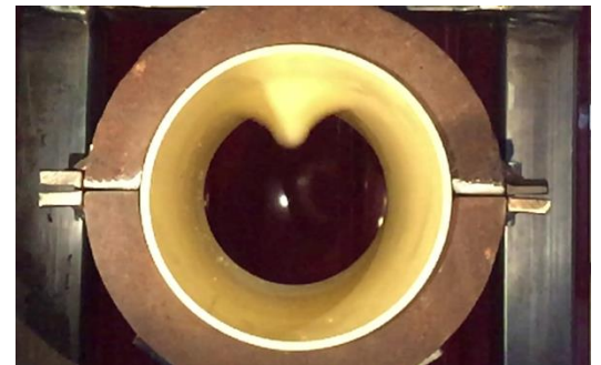
Figure 3. Deformation of the entire PVC-U segment is prevented by a thick steel jacket pipe. Brittle failure is inevitable (this has not yet occurred in this frame). The PVC can deform locally around the striker.
