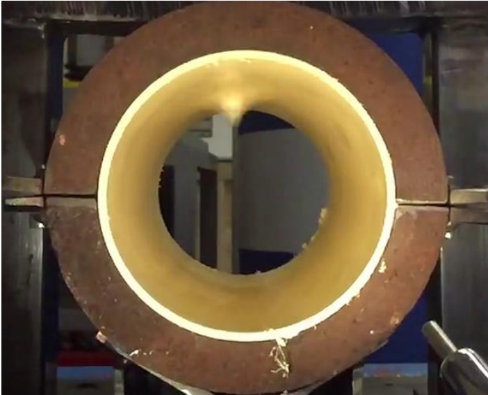
Figure 9. Still made with a high-speed camera just before failure. There is hardly any local deformation in the PVC-U pipe segment around the small striker (compare with Figure 3).
