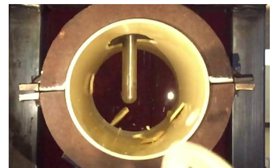
Figure 6. A few frames after Figure 3. There is local brittle failure only.
